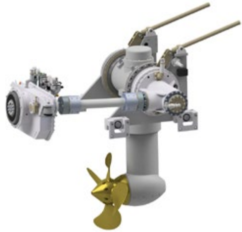
RPS – Retractable Propulsion System with the clutch box. The weight of the propulsion unit for a 286 is approx. 1200 kg and the clutch box is approx. 400 kg. The dimensions of the wet box in the hull is app. 2x1x1 m.
