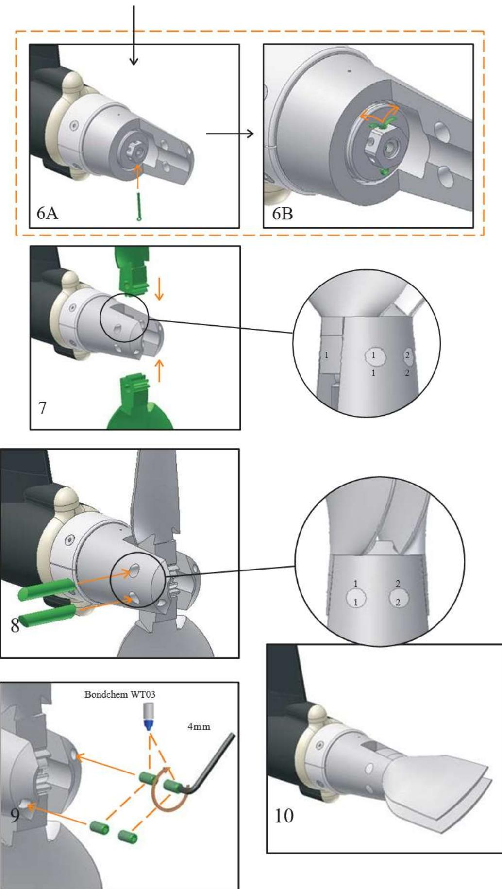
Dismount of a complete propeller for sail drive " – (B).
