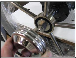
To dismount the steering wheel on a hydraulic steering system, first remove the brake spinner hub by turning it counterclockwise
