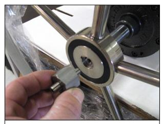
Dismount the special screw with a 24mm key, and pull of the steering wheel
