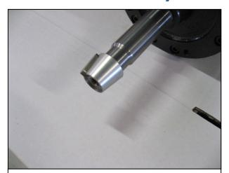
Mount your steering wheel on the shaft's conus for the wheel. Make sure the keyway in the steering wheel hub is locked with the key in steering shaft.
