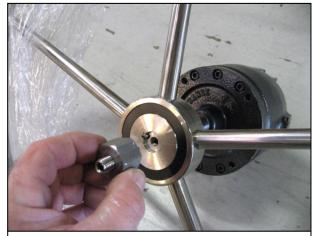
Mount the special screw, which has both a M8 thread and a M10 thread. Use the M8 thread to screw into the steering shaft, 25Nm with a 24mm key
