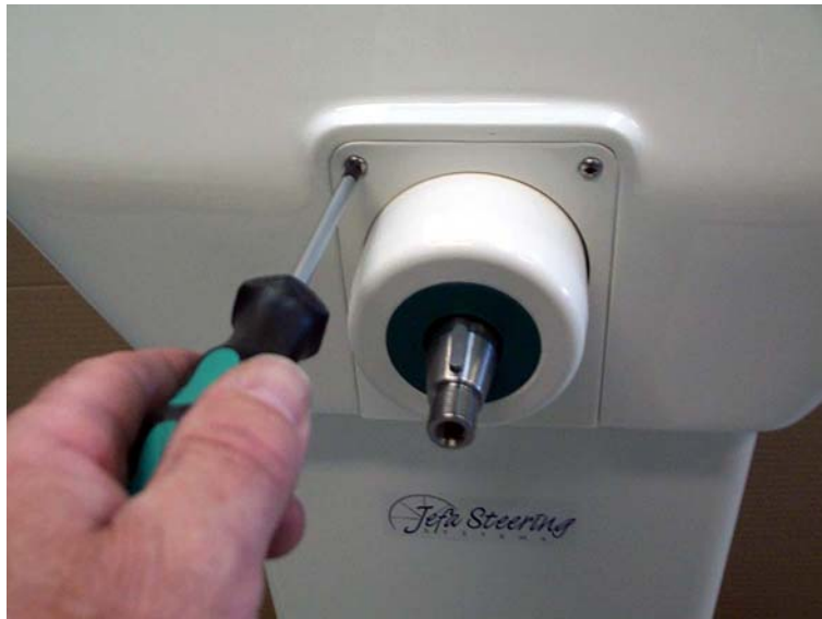
Mount the cover plate and the three screws.
