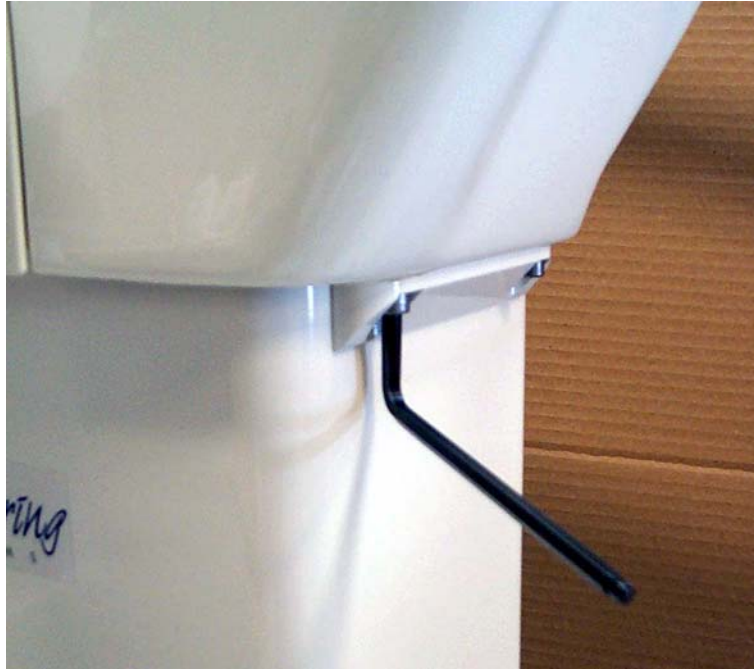
Tighten the bolts the keep the head on the pedestal.
