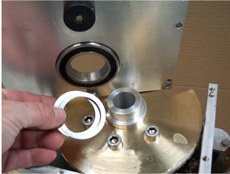
The shims that have to be put around the shaft, mostly only one shim has to be added.
