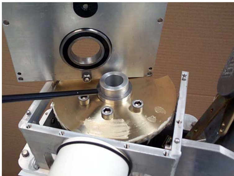
Lift off the top plate so the extra shim(s) can be added.
