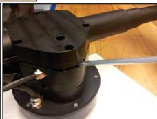
Use flat screwdriver in slid to pull housing parts from each other.
