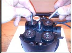
Pull out the shafts for the two front worm wheels.
