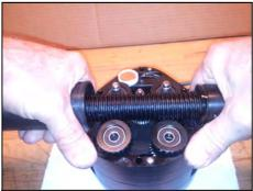
Push the back worm wheels to mount the worm shaft.
