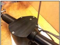
Mount bottom housing with 5pcs M6 allen screws, short one in middle.
