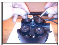
When all worm wheels are placed as described, mount the two front worm wheels with shafts.
