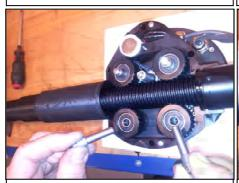
Pull out the shafts for the two back worm wheels.
