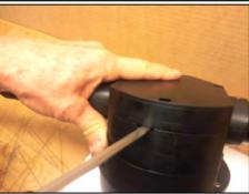
Use flat screwdriver in slid to pull housing parts from each other.
