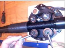
Mount the two back worm wheels with shafts.
