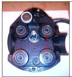
When mounting the two front worm wheels, the strait marks on the wheels have to be parallel pointing towards the center of the two back work wheels. If this is not done like this, then the worm shaft cannot be mounted, and assembly will be impossible.
