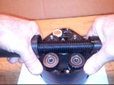
Pull the worm shaft towards the back worm wheels, and up.
