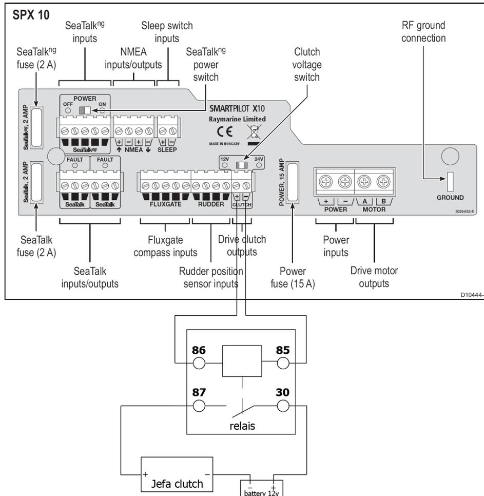
Example of the wiring diagram for the contactor.
