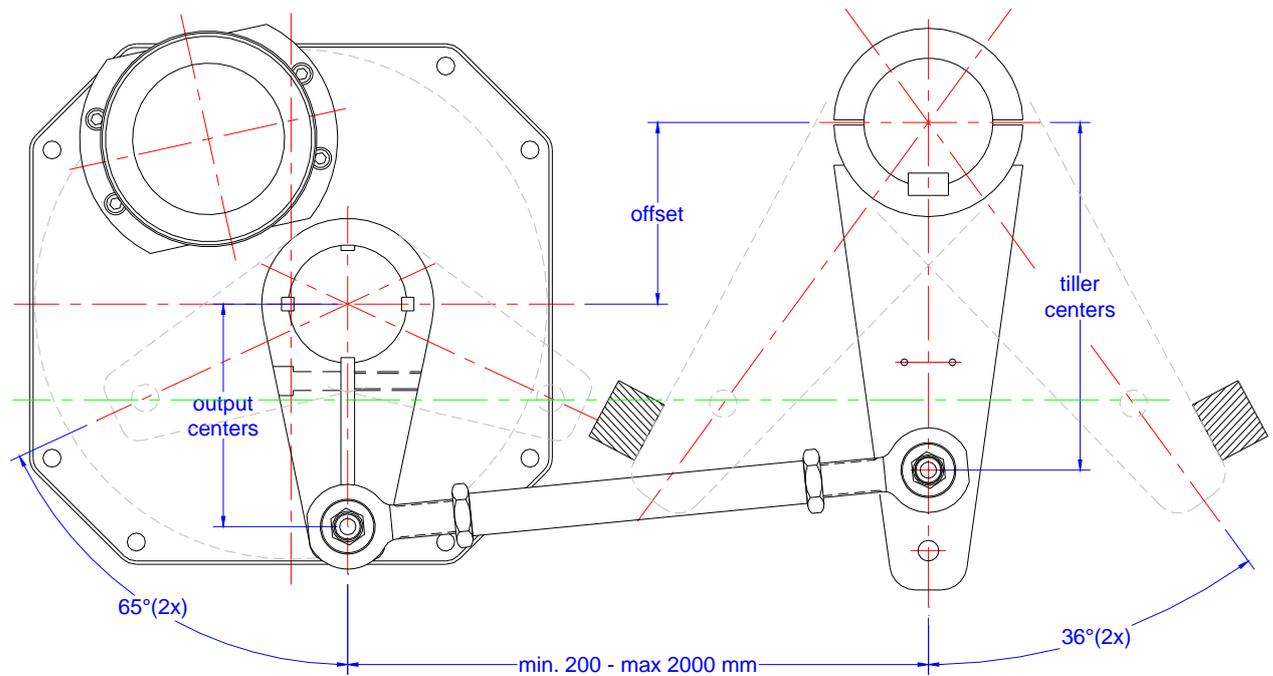
The direct drive uses “wide angle geometry”. The result of this is 128° travel of the output lever and 72° travel of the tiller lever. To achieve an equal travel of the drive in port and starboard, the centre point of the output lever needs an offset to the rudderstock centre. The offset depends on the used lever centres. Following table shows the correct offset distances:
