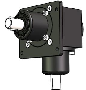
1. To remove play in your bevel box, use one 8mm allen key to dismount 4pcs screws from one input socket
